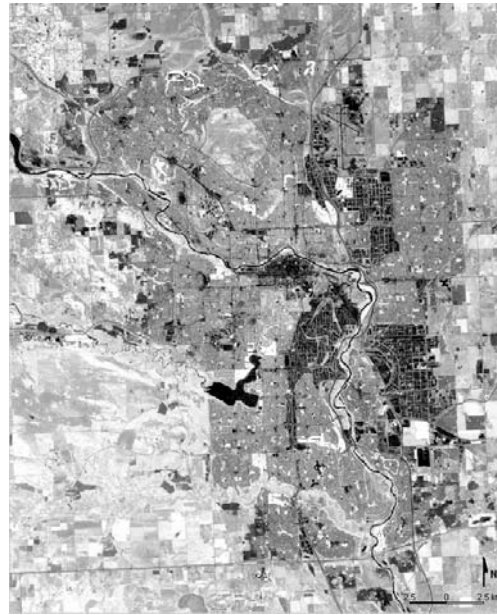
Fig. 7: NDVI (black areas within the city limits represent industrial and manufacturing land uses with black areas on the fringe indicating excavated land).
